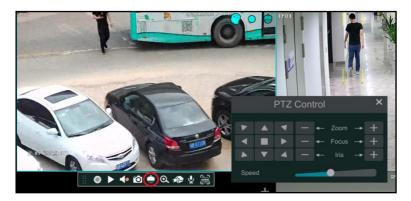
The direction, zoom, focus, iris and speed can be controlled in the small PTZ control window. Right click the PTZ/speed dome camera window and select "PTZ Control" to go to the PTZ control panel as shown below.
