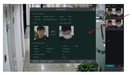
When a captured face picture is successfully recognized, click the picture on the right to open a face detail window as shown above. In this window, you can see the captured face picture, the matched picture from face library and the relevant information. You also can view the original image, search image by snapshot, play back by snapshot and export the face details by clicking "More" button.
