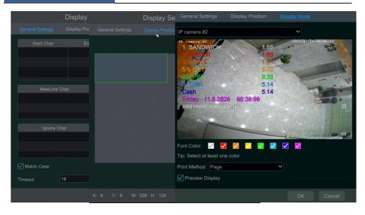
Click the "Display Color" tag and then choose the color you want to display on the screen. Multi-color can be selected at the same time. In addition, print method and preview display can be set here. If "Preview Display" is enabled, the POS contents can be displayed on the live view/playback interface.
