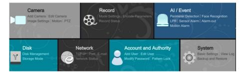
The setup panel includes seven modules. Each module provides some function entries with links for convenient operation.
