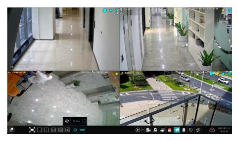
Go to the live view interface and then click it to open a small window. Set the dwell time in the window and then click it to view the live group by group according to the camera number of the current screen mode. Double click the sequence view interface to pause the view; double click again to restore the view. Click it to stop the view.
