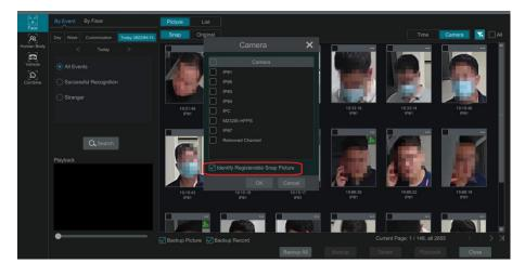
② Click T to choose face detection cameras. You can enable "Identify Registerable Snap Picture". Then the picture which can be added to the face database will be marked with a green icon.
