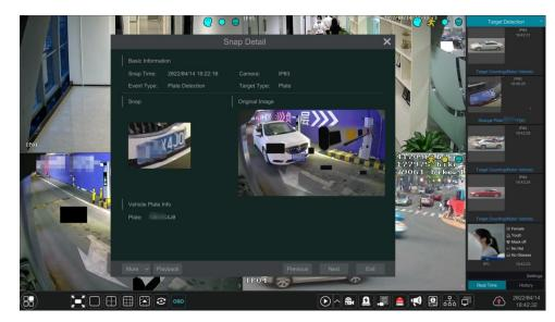
Click the captured plate picture and then it will open a detailed information window. You can view the snapshot picture, original picture, snapshot time, camera, etc. Click "More" to view the ID information of the target and export the captured picture. Click "Search" to go to the
