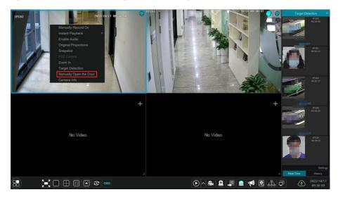
If you want to view the real-time face snapshots and comparison of access control devices, please enable face detection or comparison function as needed. Then the corresponding results will display under the target detection tab in the live interface.
