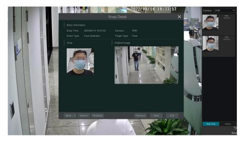
Double click a face picture to see the snapshot details, such as snapshot picture, original image, snapshot time and camera. Click "more" and then a dropdown list will display with more options. Click "Register" to register the current snapshot. Click "Search" to go to face search
