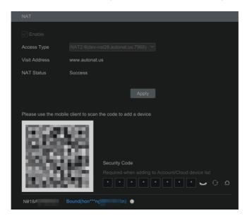
Check "Enable" and then select the NAT server address. Click "Apply" to save the settings. You can scan the QRCode through mobile APP which is installed on a mobile phone or tablet PC to quickly add the device to the server list of the mobile APP. Access Type: NAT or NAT2.0 can be selected. Click "Advanced" to select the area as needed.
